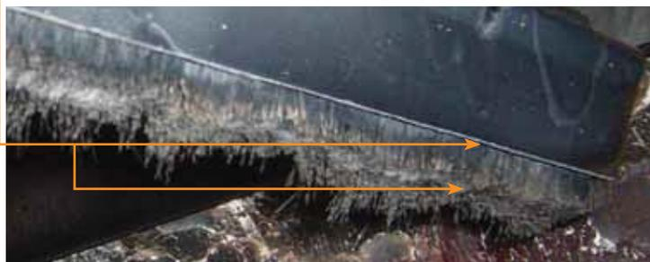
Close-up of the leading edge of the outer seal where extensive turn-down occurred. There is some brush wear, but it remains dense and provides effective sealing beyond where a strip seal would end.
